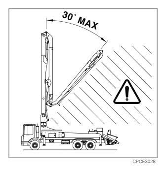
Falling-boom hazard. Do not retract boom 2 into boom 1 when unfolded.
